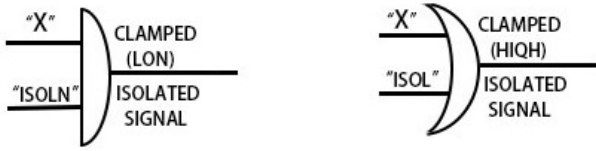
Figure 4: Isolation Cell Composed of Logic Gates.
